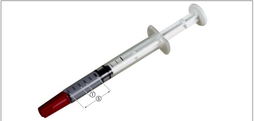
Figure 129: Measuring the thermal paste
